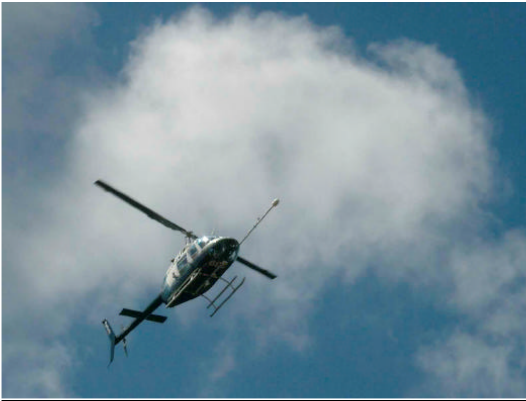
Figure 3a Helicopter with stinger instrument mount
